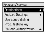
The menu structure comprises several levels. The first line in this structure shows the menu currently selected while the second line shows an option from this menu. An arrow next to an entry indicates additional options for this entry.
